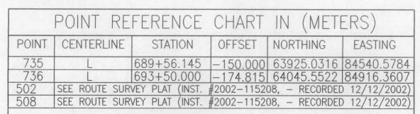
NOTE: STATIONS & OFFSETS CONTROL OVER BOTH NORTH & EAST COORDINATES AND BEARINGS AND DISTANCES. THE COORDINATE & BEARING SYSTEMS USED ON THIS CHART ARE THE SAME SYSTEMS USED ON THE ROUTE SURVEY PLAT IN INSTRUMENT #2002-115208.
