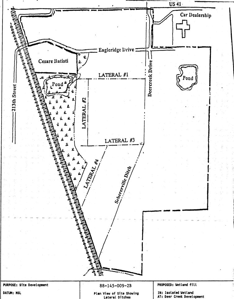
Plan View of Site Showing Lateral Ditches Scale: 1"=600'
